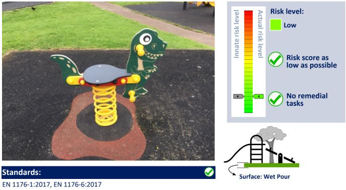
EN 1176-1:2017, EN 1176-6:2017 The item and its surfacing (where applicable) meet with the requirements of the relevant standards.
